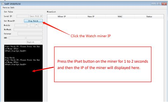
3、 Set all the miners to Static IP in a batch by configuring the IP related settings as shown in the figure below:
