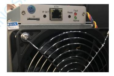
IP SET button: Press it more than 5 seconds to recover the IP to 192.168.1.25
