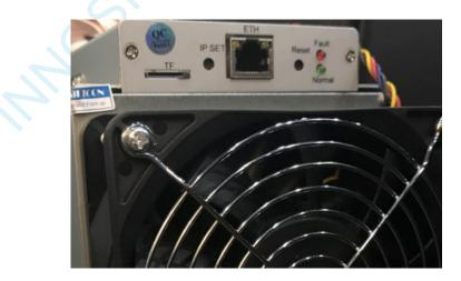
IP SET button: Press it more than 5 seconds to recover the IP to 192.168.1.25 Press it more than 20 seconds to switch the Dynamic (Static) IP to Static (Dynamic) 4. RESET button: Your miner will restart if you press it. It wont recover your settings to the default.
