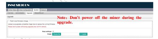
d) When you see the progress bar reach to 100%, the miner will reboot. When the reboot is done. Upgrade done. Then you can take the TF card out of the miner after press the RESET buttom
